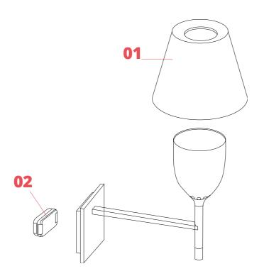
KTribe Wall & Floor 1 aluminized RF625500 bronze diffuser assembly
