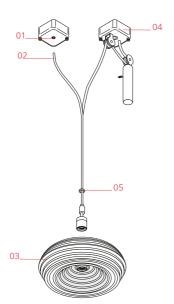
O1. Complete ceiling rose RF6500109O2. Electric wiring 2,5mt RF04637
