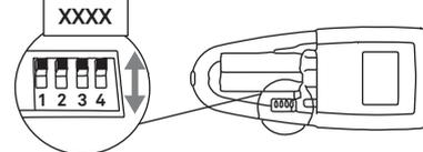
Choose the fan working frequency using the switches you can find in the remote control.
