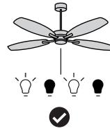
Press the button "OFF" of the remote control for 3 seconds until the light of the fan flashes. In case of fans without light you will hear a "click" when the remote control is synchronized.
