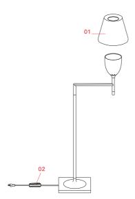
01. KTribe Wall & Floor 1 aluminized RF6255006 bronze diffuser assembly
