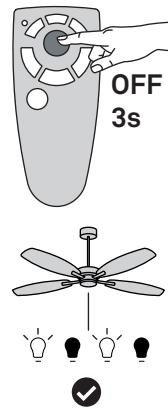
Press the button "OFF" of the remote control for 3 seconds until the light of the fan flashes. In case of fans without light you will hear a "click" when the remote control is synchronized.
