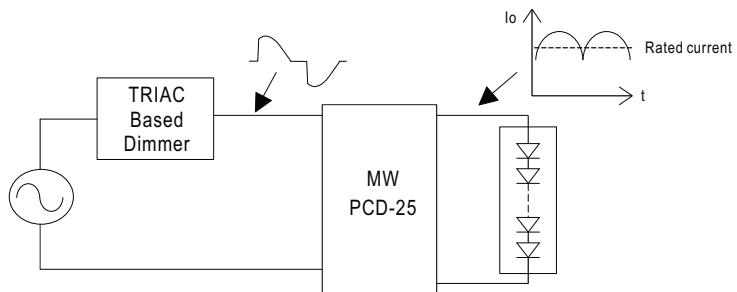
Under direct driving, the power supply will work in "constant current mode (CC)" and output voltage of the power supply will be clamped by sum of forward voltage ( $V_F$ ) of the LED strip.
